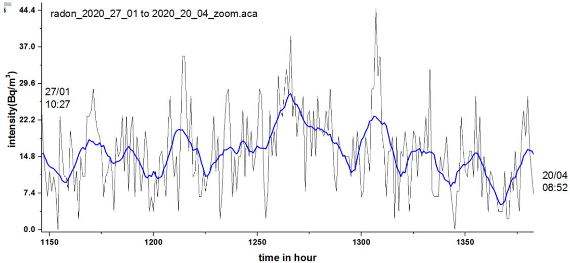
*Fig. 6 - Increased verification of the interval between measurements from 1000 to 1500 hours seen in figure 4. The variation of radon gas is observed every hour and every day*
