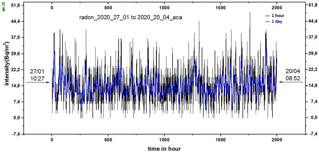
Fig. 4 – Monitoring of about 2000-hour series from Radon Eye RD200 in ACA tower using (Bq/m<sup>3</sup>) unit. The blue curves corresponding smoothed values in one day
